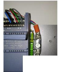
Important: The usage of a shield connector is highly recommended to avoid EMC interferences!
